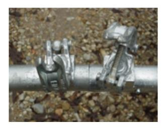
Note: All tubing is 1.90 diameter, 11-gauge (0.120 wall), high-strength, minimum 65,000 yield, and 75,000 tensile. Diagonal pin braces are designed to be compatible with standard 1.90 OD tube and clamp material.
