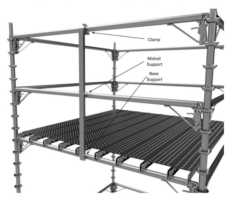
The proper way to attach a horizontal tie-off support to the horizontals is in the center of the horizontal with the clamp attached to the handrail. The clamp should slide over the handrail and the bolt should be at the bottom of the horizontal.
