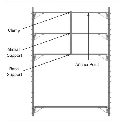
The horizontal tie-off support is designed so the horizontal bars it is connected to share the load. The single clamp design allows for the greatest amount of support with the fastest possible installation time.
