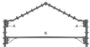
Support must be added at point "A" or "B" to prevent the verticals from spreading apart.
