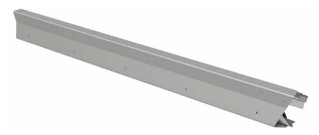
The aluminum toe board, with locking clips, is designed to fit all types of scaffold material. The toe board locks the scaffold boards down—eliminating the need to wire boards to the horizontals. Installation times are greatly reduced with this equipment.
