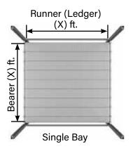
Standard board layout using the side bracket cantilever as the bearer.
