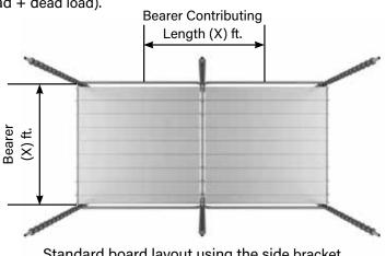
Standard board layout using the side bracket cantilever as the bearer.
